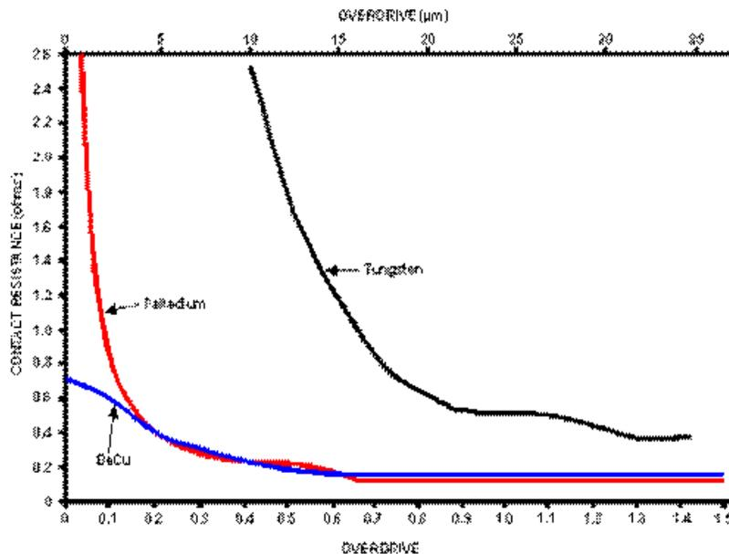
Accuprobe does not offer a Palladium alloy tip because of the difficulty maintaining planarity with this material. There is clearly a relationship of contact resistance to overdrive as discussed earlier,
